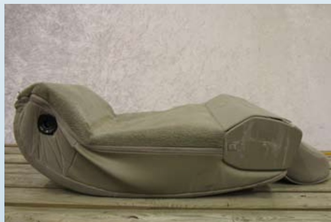
A typical dog crate made of steel tubes will easily snap the backrest in a Volvo V70.
